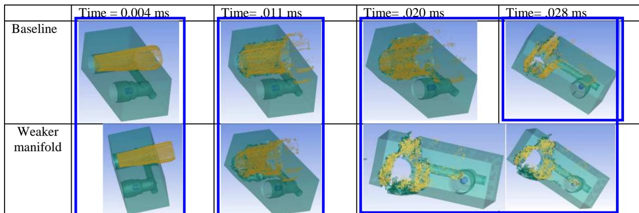
**Figure 7. Comparison of baseline and weaker manifold damage conditions at various timing.**
