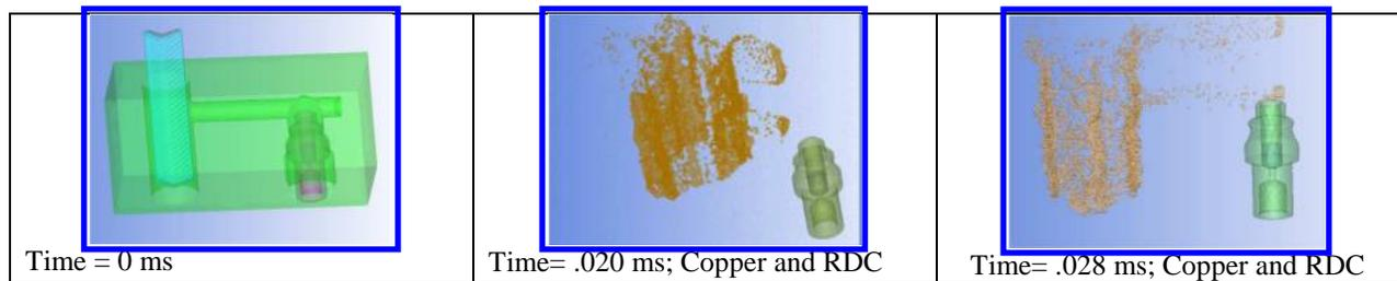
**Figure 5. FEA model and LSC liner deployment**
