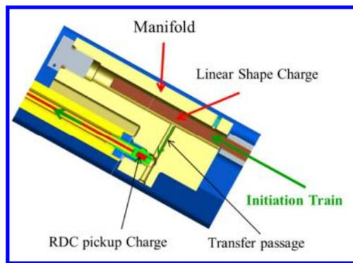
Figure 2. Cross-sectional illustration of LSC/ RDC initiation train.
