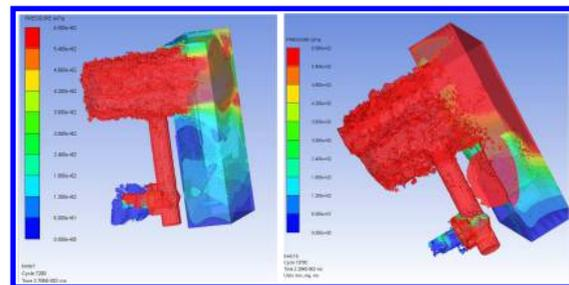
**Figure 8. Comparison of pressure profiles of PBX reaction products between baseline (left) and weaker manifold (left)**
